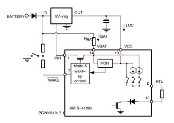
Figure 2. Connection via R<sub>BAT</sub> to V<sub>BAT</sub> Indication of Currents
