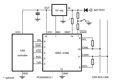
Figure 3. Single V<sub>CC</sub> Topology for 5 V Microcontroller
