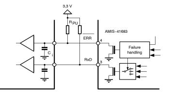
Figure 1. Pullup Resistor to Interface with True 3.3 V Microcontrollers
